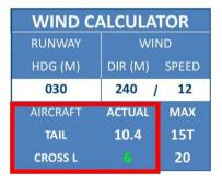
The wind components are displayed at the left lower corner of the wind calculator.
